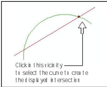
Figure 3 Line - Curve Intersection
