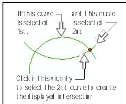
Figure 6 Curve - Curve Intersection
