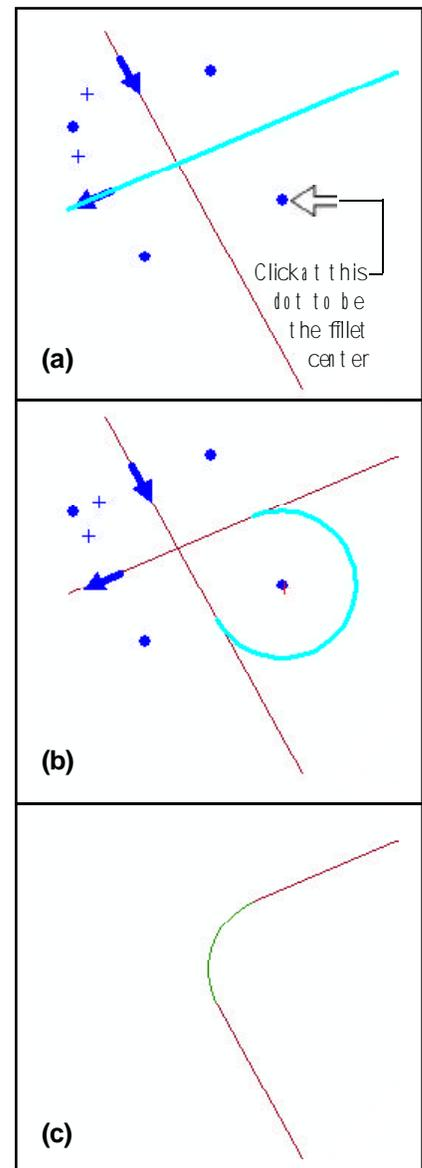
Figure 14 Introduction Of An Arc Fillet
