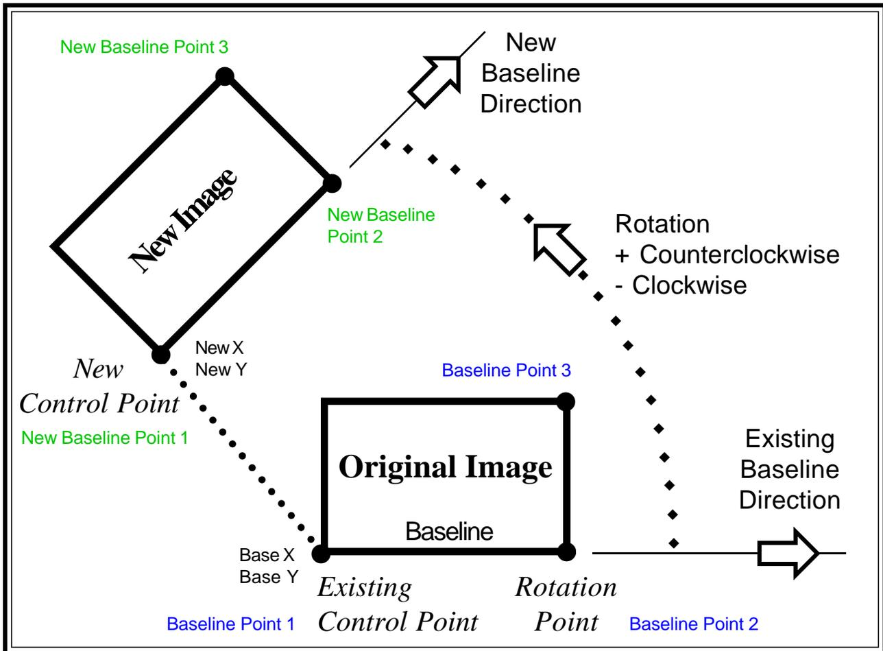
Figure 3 - Transformation Tool Control Point Locations
